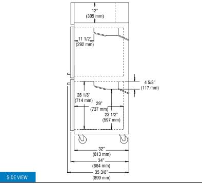
**IMPORTANT NOTE:** If the cabinet is located directly against a wall and/or under a low ceiling, a <u>minimum clearance of 12" is required</u>.
