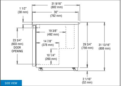
**NOTE:** For proper operation, the area under and in front of the cabinet **must** not be obstructed in any way.
