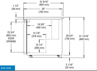
NOTE: For proper operation, the area under and in front of the cabinet must not be obstructed in any way.
