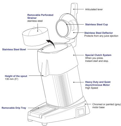
For all fruits (citrus fruits must be peeled). Continuous juice production by centrifugal action and automatic pulp ejection.
