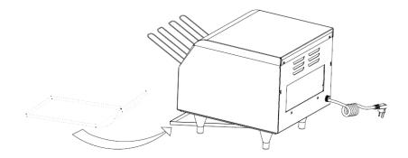
2. Put the back-cover-board to the hook in back open to block the heat outside.
