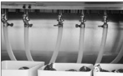
Convenient hand key screw clamps make hose removal and cleaning easy.
