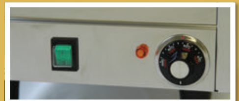
Covered master switch and adjustable thermostat
