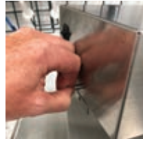
Pulling locking spring pin out to unlock the back of the lid
