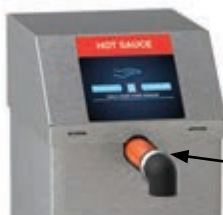
Pump primed with food product seen in discharge tube.
