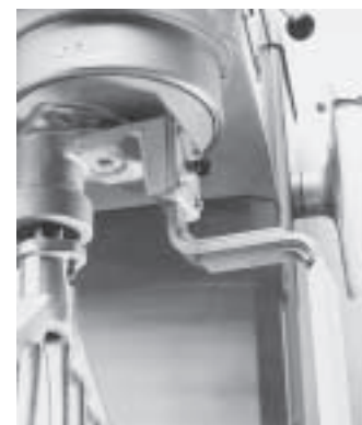
Bowl Scraper continuously scrapes side of bowl while mixing
