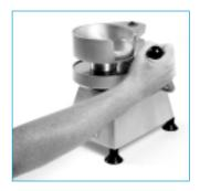
2. Press release button to lower press plate into forming dish. Pull handle forward and apply light pressure.
