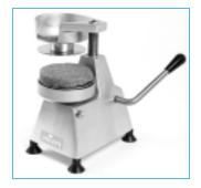
3. Return handle to the rear. Press plate rises automatically for easy removal.
