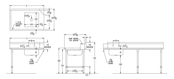
All units ship unassembled for reduced shipping cost. Units 7 ft. and larger are furnished with four legs. All dimensions are typical. Tolerance +/- .500".
