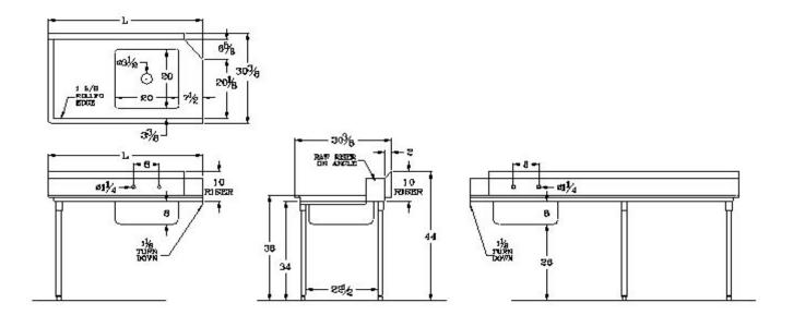
All units ship unassembled for reduced shipping cost. Units 7 ft. and larger are furnished with four legs. All dimensions are typical.
