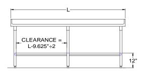
All units ship unassembled for reduced shipping cost. Units 7 ft. and larger are furnished with six legs. All dimensions are typical.
