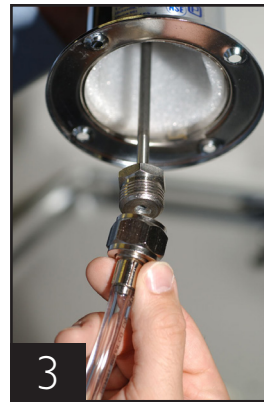
3 Thread beer line connector to draft arm and secure draft arm to cabinet with rubber gasket under the draft arm.
