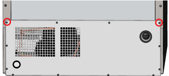
Fig. 2. For the TFP (a closed-back unit), remove the indicated screws to install the shelf supports.
