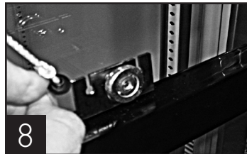
Door roller bracket with nylon cord.
