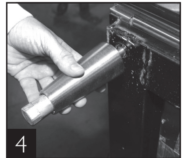
4 Thread leg into cabinet bottom frame rail.
