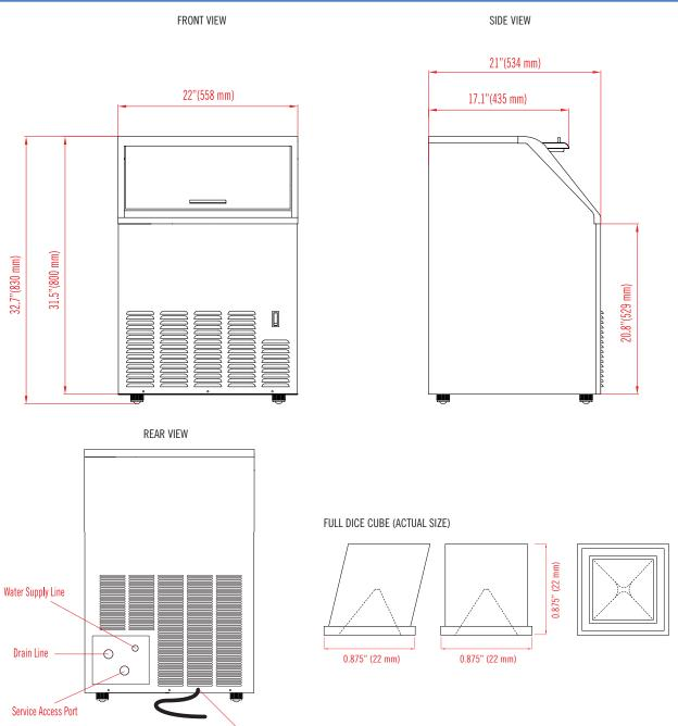
DAILY ICE BIN STORAGE NET WEIGHT / AMP DRAW REFRIGERANT EXTERNAL MODEL ICE PRODUCTION ELECTRICAL DIMENSIONS SHIPPING WEIGHT (MAKING / HARVESTING) AND CHARGE SIZE CAPACITY (70°F Air / 50°F Water) 22" x 21" x 32.7" 110 lbs (50 kg) R-134a 69K-904 120 lbs (54.4 kg) 35 lbs (15.9kg) 7.5A / 11.8A 115V / 60Hz / 1Ph (558 x 534 x 830 mm) 129 lbs (58.5 kg) 8.47oz (240g)
