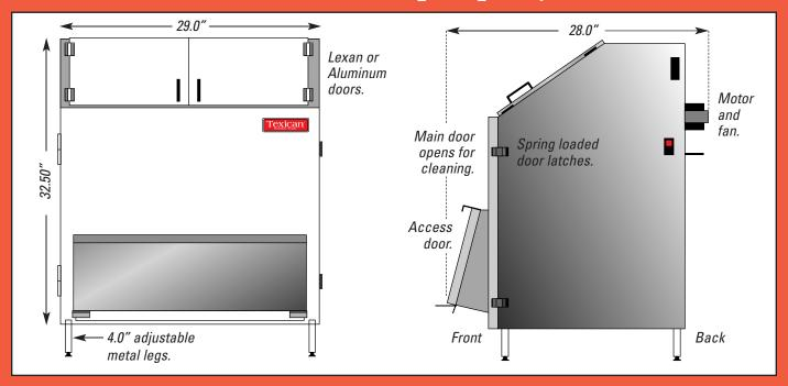
Option: .250 thick anodized aluminum loading doors.
