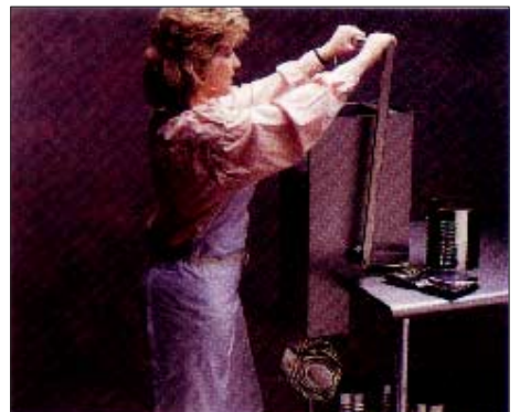
Return handle to upright position. Crushed can falls into receptacle.
