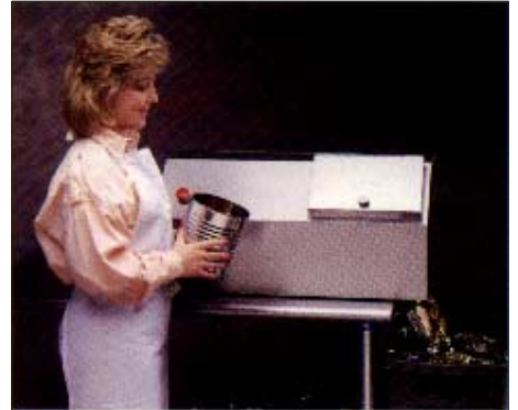
Crushed can falls into receptacle.
