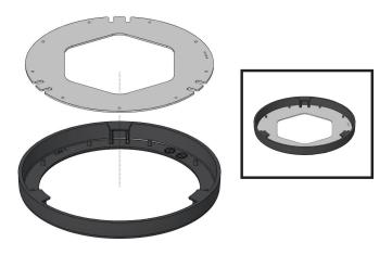
6. REPLACE COVER RING WITH GASKET BY TURNING CLOCKWISE OVER MOUNTING RING UNTIL SECURE
