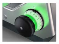
Green means motor off gauge plate closed.
