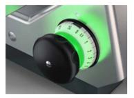
Green means motor off gauge plate closed.
