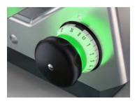
Green means motor off gauge plate closed.
