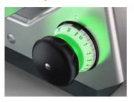
Green means motor off gauge plate closed.
