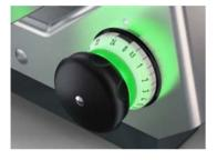
Green means motor off gauge plate closed.
