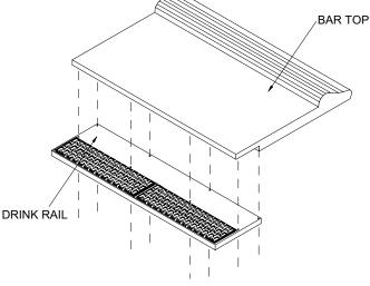
Apply silicone sealant to the rear mounting surface of the drink rail. Install unit by securing to underside of bar top with wood screws provided. If installing to material other than wood, use appropriate screws to secure. Plumb drain once installed.
