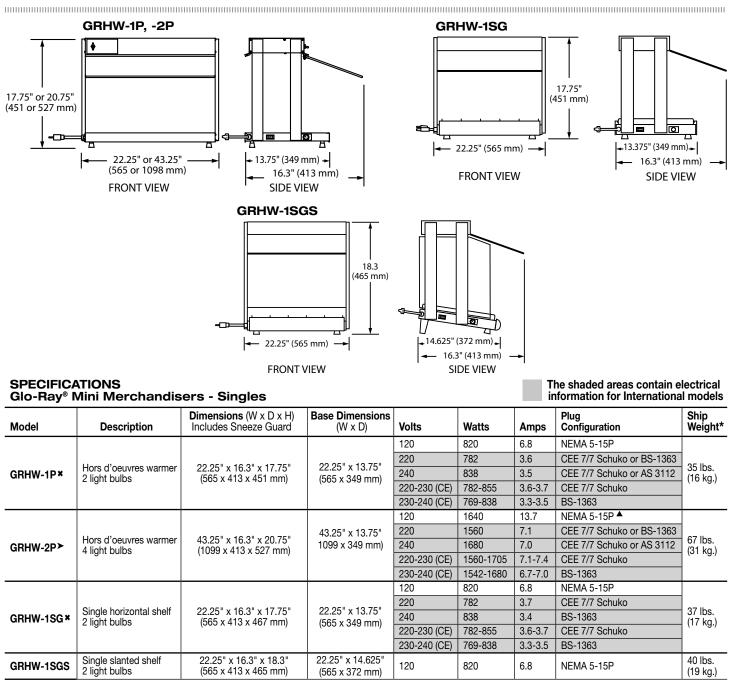
\* Shipping weight includes packaging. \*Add 3" (76 mm) to height when using accessory 4" (102 mm) legs. ≻ Standard 4" (102 mm) legs included in height. A NEMA 5-20P for Canada.
