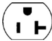
20 Amp Outlet For 120V 2000 Watt Cabinets
