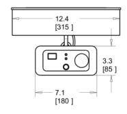
Range Glass Cut Out 13.5" L x 12.625" W 342 mm L x 322 mm W Contol Panel Cutout 5.75" L x 2.71" W 146 mm L x 69 mm W
