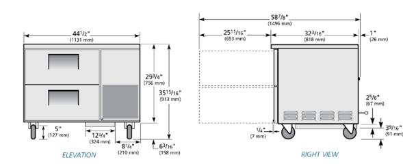
WARRANTY\* Three year warranty on all parts and labor and an additional 2 year METRIC DIMENSIONS ROUNDED UP TO THE NEAREST WHOLE MILLIMETER Model Elevation Right Plan ЗD Back warranty on compressor. (U.S.A. only) ксі TUC-44D-2 TFPY65E TFPY65S TFPY65P TFPY653 SPECIFICATIONS SUBJECT TO CHANGE RESIDENTIAL APPLICATIONS: TRUE assumes no liability for parts or labor coverage for component failure or other damages resulting from installation in non-commercial or residential applications. WITHOUT NOTICE
